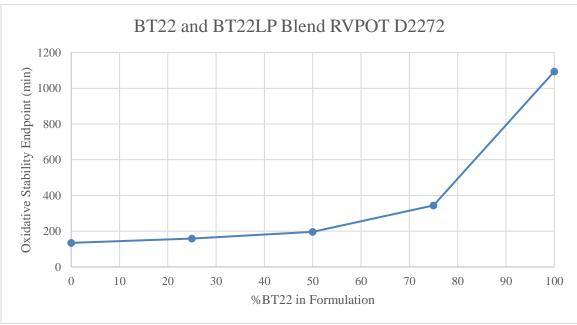
Graph 2 - Plot of Oxidative Stability versus Percent BT22 in 2 Component Blend
